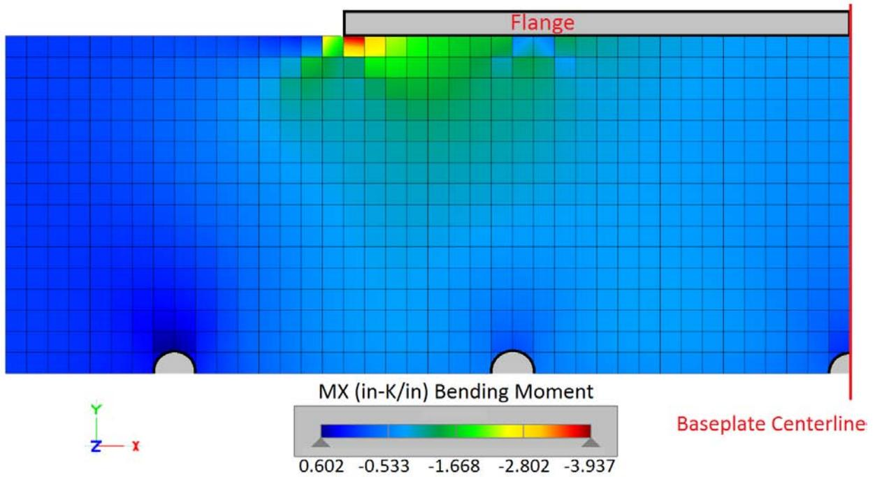
Figure 6: Connection B (five bolts) MX Bending
