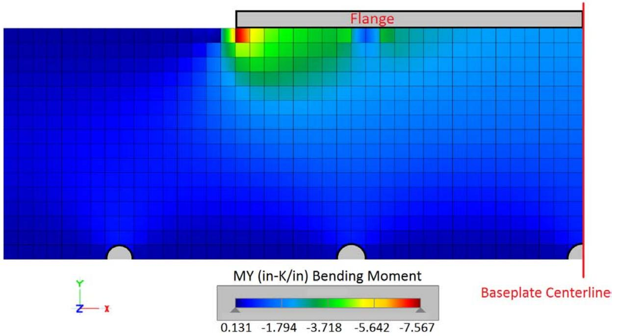
Figure 5: Connection B (five bolts) MY Bending
