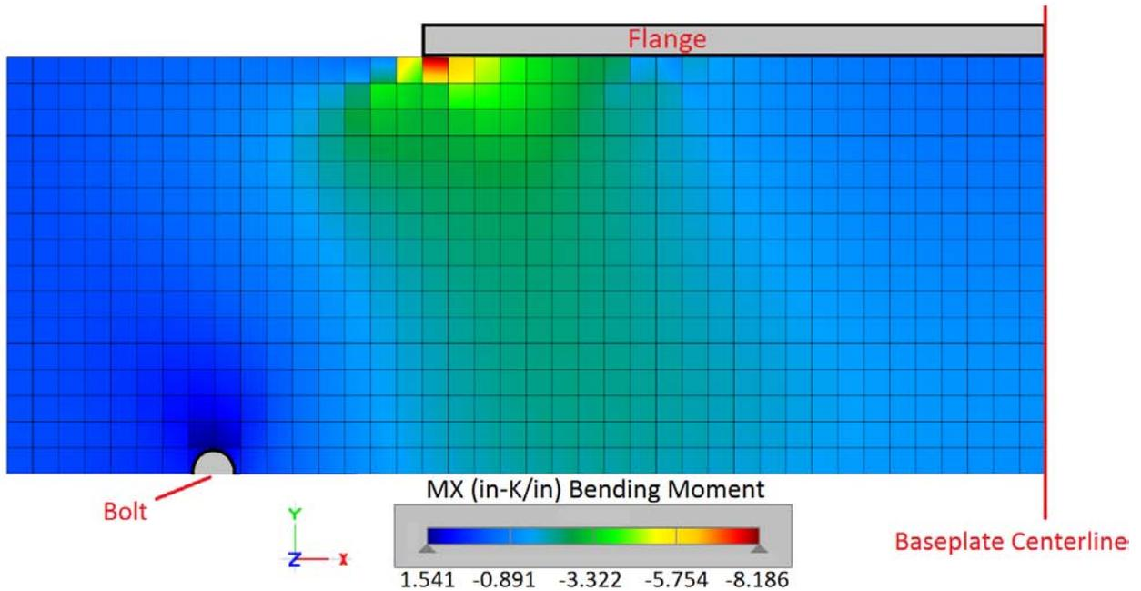
Figure 4: Connection A (two bolts) MX Bending
