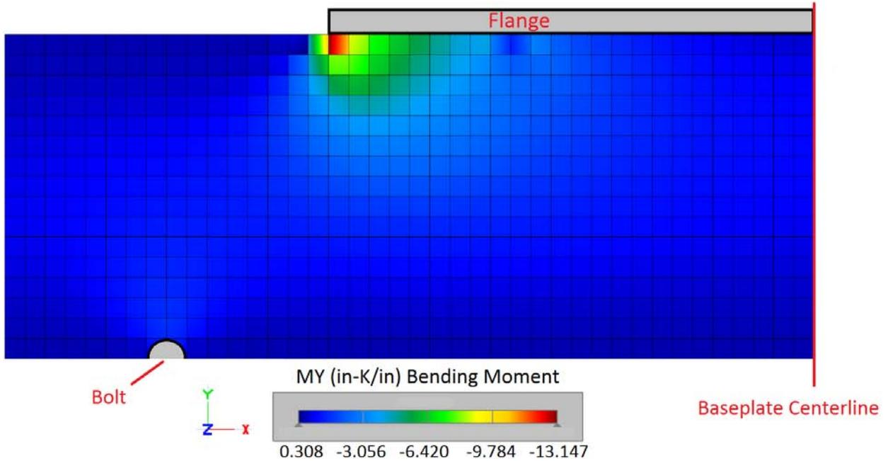
Figure 3: Connection A (two bolts) MY Bending
