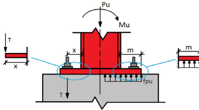
Figure 1: DG1 Base Plate Bending Models
